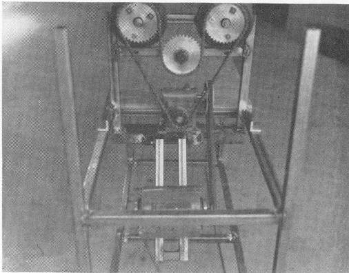
FIG. 3. Driving mechanism for modified rotary sieve. One-fourth horsepower electric motor, 24:1 speed reducer, roller chain, and drive wheels.
