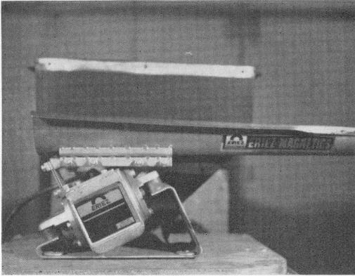
FIG. 2. Vibratory feeder with 3 by 20-inch half-round tray and a 0- to 2-ton-per-hour feeding rate. Model 20A Eriez Magnetics<sup>®</sup>, Erie, Pennsylvania.
