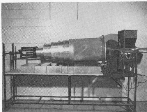
FIG 1. Modified rotary sieve, side view.
